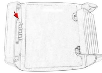
2、 Rechargeable contacts are connected to the charging interface of the tracker and The mobile power supply is mounted on the tracker.
